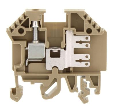
Feed-through terminal, Faston Spade connection / screw connection, Mounting type:Mounting rail TS 35/7.5 and TS 32, Rated cross-section: 2.5 mm², Width: 6 mm, Colour: Beige
