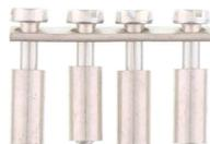
Cross-connector, No. of poles: 4, Mounting type: Can be screwed on, Width: 22.7 mm, Rated cross-section: 4 mm<sup>2</sup>, Colour: natural
