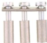
Cross-connector, No. of poles: 3, Mounting type: Can be screwed on, Width: 16.6 mm, Rated cross-section: 4 mm<sup>2</sup>, Colour: natural
