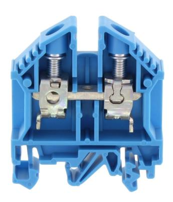
Feed-through terminal, Screw connection, Mounting type:Mounting rail TS 35/7.5 and TS 32, Rated cross-section: 16 mm², Width: 12 mm, Colour: Blue
