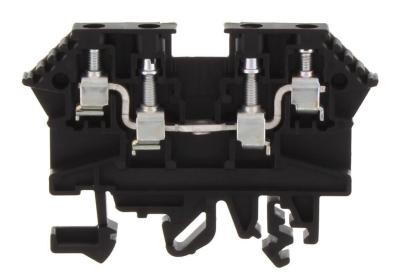
Feed-through terminal, Screw connection, Mounting type:Mounting rail TS 35/7.5 and TS 32, Rated cross-section: 4 mm², Width: 6 mm, Colour: Black
