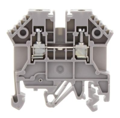
Feed-through terminal, Screw connection, Mounting type:Mounting rail TS 35/7.5 and TS 32, Rated cross-section: 2.5 mm², Width: 5 mm, Colour: Grey
