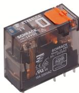
Plug-in industrial relays with power contacts, 1 CO contact, Test button, Status LED, Free-wheel diode, Mechanical switching position indicator, Polarity A1+, A2-, Input voltage: 24 VDC
