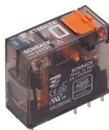
Plug-in industrial relays with power contacts, 1 CO contact, Test button, Status LED, Mechanical switching position indicator, Input voltage: 24 VAC
