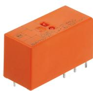
Plug-in miniature power relay, Encapsulated design with power contact, 1 CO contact, Input voltage: 24 VDC
