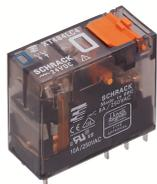
Plug-in industrial relays with power contacts, 2 CO contacts, Test button, Status LED, Mechanical switching position indicator, Input voltage: 24 VAC
