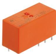
Plug-in miniature power relay, Encapsulated design with power contact, 2 CO contacts, Input voltage: 24 VAC
