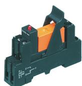
Pre-assembled relay module PRS..., Screw connection, Consisting of: relay socket base, power contact relay, pluggable display/suppression module and holding clip, 1 CO contact, Input voltage: 110 VDC
