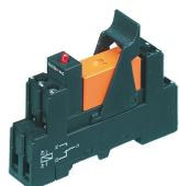
Pre-assembled relay module PRS..., Screw connection, Consisting of: relay socket base, power contact relay, pluggable display/suppression module and holding clip, 1 CO contact, Input voltage: 12 VDC
