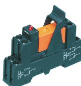
Pre-assembled relay module PRS..., Screw connection, Consisting of: relay socket base, power contact relay, pluggable display/suppression module and holding clip, 2 CO contacts, Input voltage: 110 VDC
