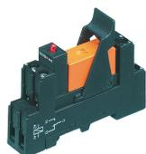
Pre-assembled relay module PRS..., Screw connection, Consisting of: relay socket base, power contact relay, pluggable display/suppression module and holding clip, 1 CO contact, Input voltage: 5 VDC
