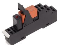
Pre-assembled relay module PRS..., Tension-spring connection, Consisting of: relay socket base, power contact relay, pluggable display/suppression module and holding clip, 1 CO contact, Input voltage: 60 VDC
