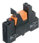
Pre-assembled relay module PRS..., Screw connection, Consisting of: relay socket base, power contact relay, pluggable display/suppression module and holding clip, 2 CO contacts, Input voltage: 230 VAC
