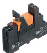
Pre-assembled relay module PRS..., Screw connection, Consisting of: relay socket base, power contact relay, pluggable display/suppression module and holding clip, 2 CO contacts, Input voltage: 115 VAC
