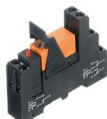
Pre-assembled relay module PRS..., Screw connection, Consisting of: relay socket base, power contact relay, pluggable display/suppression module and holding clip, 2 CO contacts, Input voltage: 12 VDC
