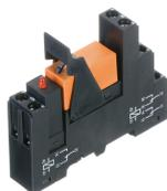
Pre-assembled relay module PRS..., Screw connection, Consisting of: relay socket base, power contact relay, pluggable display/suppression module and holding clip, 2 CO contacts, Input voltage: 230 VAC
