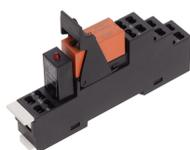
Pre-assembled relay module PRS..., Tension-spring connection, Consisting of: relay socket base, power contact relay, pluggable display/suppression module and holding clip, 2 CO contact, Input voltage: 115 VAC
