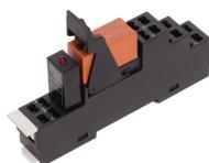
Pre-assembled relay module PRS..., Tension-spring connection, Consisting of: relay socket base, power contact relay, pluggable display/suppression module and holding clip, 1 CO contact, Input voltage: 230 VAC
