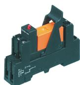
Pre-assembled relay module PRS..., Screw connection, Consisting of: relay socket base, power contact relay, pluggable display/suppression module and holding clip, 1 CO contact, Input voltage: 115 VAC
