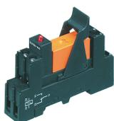
Pre-assembled relay module PRS..., Screw connection, Consisting of: relay socket base, power contact relay, pluggable display/suppression module and holding clip, 1 CO contact, Input voltage: 24 VAC
