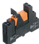
Pre-assembled relay module PRS..., Screw connection, Consisting of: relay socket base, power contact relay, pluggable display/suppression module and holding clip, 2 CO contacts, Input voltage: 24 VAC
