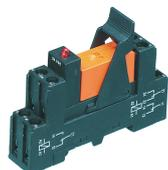
Pre-assembled relay module PRS..., Screw connection, Consisting of: relay socket base, power contact relay, pluggable display/suppression module and holding clip, 2 CO contacts, Input voltage: 12 VDC
