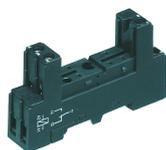
Relay socket base PRS, for miniature power relay with 1 CO contact, Screw connection, Plug-in option for input/suppression modules, Mounting type: Mounting rail TS 35
