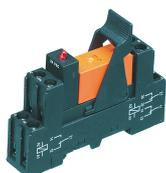
Pre-assembled relay module PRS..., Screw connection, Consisting of: relay socket base, power contact relay, pluggable display/suppression module and holding clip, 2 CO contacts, Input voltage: 48 VDC
