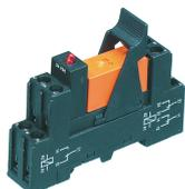
Pre-assembled relay module PRS..., Screw connection, Consisting of: relay socket base, power contact relay, pluggable display/suppression module and holding clip, 2 CO contacts, Input voltage: 24 VAC
