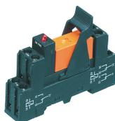
Pre-assembled relay module PRS..., Screw connection, Consisting of: relay socket base, power contact relay, pluggable display/suppression module and holding clip, 2 CO contacts, Input voltage: 12 VDC
