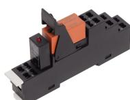
Pre-assembled relay module PRS..., Tension-spring connection, Consisting of: relay socket base, power contact relay, pluggable display/suppression module and holding clip, 2 CO contact, Input voltage: 24 VDC
