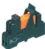
Pre-assembled relay module PRS..., Screw connection, Consisting of: relay socket base, power contact relay, pluggable display/suppression module and holding clip, 1 CO contact, Input voltage: 12 VDC
