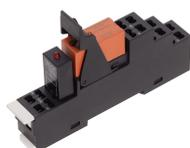
Pre-assembled relay module PRS..., Tension-spring connection, Consisting of: relay socket base, power contact relay, pluggable display/suppression module and holding clip, 1 CO contact, Input voltage: 115 VAC
