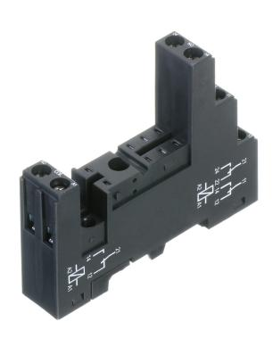
Relay socket base PRS, for miniature power relay with 2 CO contacts, Screw connection, Plug-in option for input/suppression modules, Mounting type: Mounting rail TS 35
