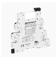
Interface-Relay-Compact (IRC) Complete, Consisting of base FIRCU... with Push-In connection and pluggable miniature relay with power contact, Mounting type: Mounting rail TS 35, 1 CO contact, Input voltage: 6 VAC/DC
