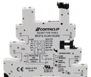
Interface-Relay-Compact (IRC) socket base IRC with screw connection, Mounting type: Mounting rail TS 35, 1 CO contact, Input voltage: 6, 12 or 24 VAC/DC
