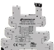
Interface-Relay-Compact (IRC) socket base FIRC I with Push-In connection, Mounting type: Mounting rail TS 35, 1 CO contact, Input voltage: 6 to 24 VAC/DC
