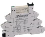
Plug-Relay-Compact (PRC) Complete, Consisting of base PRC... with screw connection and pluggable miniature relay PRC... with power contact, Mounting type: Mounting rail TS 35, 1 CO contact, Input voltage: 6 VDC
