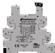
Interface-Relay-Compact (IRC) socket base IRCO with screw connection, Mounting type: Mounting rail TS 35, 1 CO contact, Input voltage: 6, 12 or 24 VAC/DC
