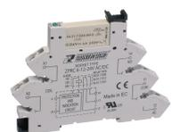
Plug-Relay-Compact (PRC) socket base PRC with tension-spring connection, Mounting type: Mounting rail TS 35, 1 CO contact, Input voltage: 6, 12 or 24 VDC
