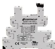
Interface-Relay-Compact (IRC) socket base IRCI with screw connection, Mounting type: Mounting rail TS 35, 1 CO contact, Input voltage: 6 to 24 VAC/DC
