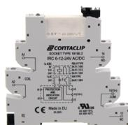
Interface-Relay-Compact (IRC) Complete, Consisting of base IRC... with screw connection and pluggable miniature relay PRC... with power contact, Mounting type: Mounting rail TS 35, 1 CO contact, Input voltage: 6 VAC/DC
