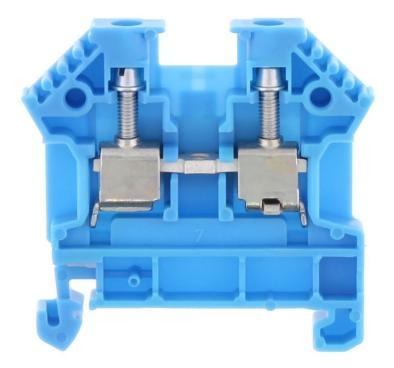
Feed-through terminal, Screw connection, Mounting type: Mounting rail TS 35/7.5, Rated cross-section: 4 mm<sup>2</sup>, Width: 6 mm, Colour: Blue
