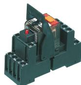
Pre-assembled relay module PRSU..., Screw connection, Consisting of: relay socket base, power contact relay, pluggable display/suppression module and holding clip, 4 CO contacts, Input voltage: 220 VDC
