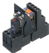
Pre-assembled relay module PRSU..., Screw connection, Consisting of: relay socket base, power contact relay, pluggable display/suppression module and holding clip, 4 CO contacts, Input voltage: 230 VAC
