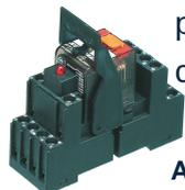
Pre-assembled relay module PRS..., Screw connection, Consisting of: relay socket base, power contact relay, pluggable display/suppression module and holding clip, 4 CO contacts, Input voltage: 48 VDC
