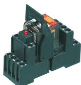
Pre-assembled relay module PRSU..., Screw connection, Consisting of: relay socket base, power contact relay, pluggable display/suppression module and holding clip, 4 CO contacts, Input voltage: 48 VDC
