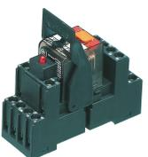
Pre-assembled relay module PRSU..., Screw connection, Consisting of: relay socket base, power contact relay, pluggable display/suppression module and holding clip, 4 CO contacts, Input voltage: 24 VAC
