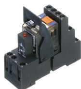
Pre-assembled relay module PRSU..., Screw connection, Consisting of: relay socket base, power contact relay, pluggable display/suppression module and holding clip, 4 CO contacts, Input voltage: 48 VDC
