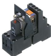
Pre-assembled relay module PRSU..., Screw connection, Consisting of: relay socket base, power contact relay, pluggable display/suppression module and holding clip, 4 CO contacts, Input voltage: 24 VAC
