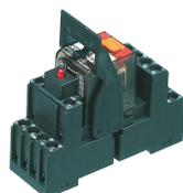
Pre-assembled relay module PRSU..., Screw connection, Consisting of: relay socket base with multi-layer gold contact, pluggable display/suppression module and holding clip, 4 CO contacts, Input voltage: 24 VDC
