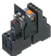
Pre-assembled relay module PRSU..., Screw connection, Consisting of: relay socket base, power contact relay, pluggable display/suppression module and holding clip, 4 CO contacts, Input voltage: 220 VDC
