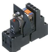
Pre-assembled relay module PRSU..., Screw connection, Consisting of: relay socket base, power contact relay, pluggable display/suppression module and holding clip, 4 CO contacts, Input voltage: 24 VDC
