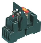
Pre-assembled relay module PRS..., Screw connection, Consisting of: relay socket base, power contact relay, pluggable display/suppression module and holding clip, 4 CO contacts, Input voltage: 220 VDC
