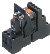
Pre-assembled relay module PRS..., Screw connection, Consisting of: relay socket base, power contact relay, pluggable display/suppression module and holding clip, 4 CO contacts, Input voltage: 12 VDC
