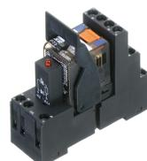
Pre-assembled relay module PRS..., Screw connection, Consisting of: relay socket base, power contact relay, pluggable display/suppression module and holding clip, 4 CO contacts, Input voltage: 115 VAC
