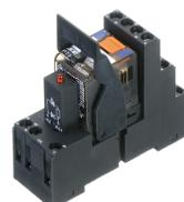
Pre-assembled relay module PRS..., Screw connection, Consisting of: relay socket base, power contact relay, pluggable display/suppression module and holding clip, 4 CO contacts, Input voltage: 48 VDC
