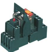
Pre-assembled relay module PRSU..., Screw connection, Consisting of: relay socket base, power contact relay, pluggable display/suppression module and holding clip, 4 CO contacts, Input voltage: 12 VDC
