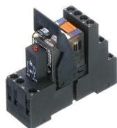
Pre-assembled relay module PRSU..., Screw connection, Consisting of: relay socket base, power contact relay, pluggable display/suppression module and holding clip, 4 CO contacts, Input voltage: 12 VDC
