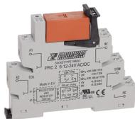
Plug-Relay-Compact (PRC) Complete, Consisting of base PRC... with screw connection and pluggable miniature relay PRS... with power contact, Mounting type: Mounting rail TS 35, 2 CO contacts, Input voltage: 240 VAC/DC
