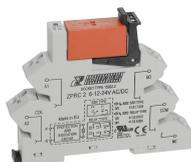
Plug-Relay-Compact (PRC) Complete, Consisting of base PRC... with tension-spring connection and pluggable miniature relay PRS... with inrush power contact, Mounting type: Mounting rail TS 35, 1 CO contact, Input voltage: 24 VAC/DC
