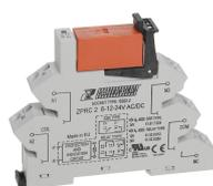
Plug-Relay-Compact (PRC) Complete, Consisting of base PRC... with tension-spring connection and pluggable miniature relay PRS... with power contact, Mounting type: Mounting rail TS 35, 2 CO contacts, Input voltage: 240 VAC/DC
