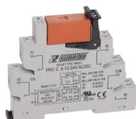
Plug-Relay-Compact (PRC) Complete, Consisting of base PRC... with screw connection and pluggable miniature relay PRS... with power contact, Mounting type: Mounting rail TS 35, 2 CO contacts, Input voltage: 24 VAC/DC
