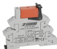
Plug-Relay-Compact (PRC) socket base PRC with tension-spring connection, Mounting type: Mounting rail TS 35, 2 CO contact, Input voltage: 220 to 240 VAC/DC
