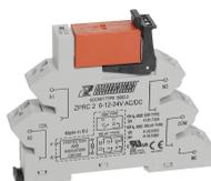
Plug-Relay-Compact (PRC) Complete, Consisting of base PRC... with tension-spring connection and pluggable miniature relay PRS... with power contact, Mounting type: Mounting rail TS 35, 2 CO contacts, Input voltage: 12 VAC/DC
