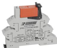
Plug-Relay-Compact (PRC) Complete, Consisting of base PRC... with tension-spring connection and pluggable miniature relay PRS... with power contact, Mounting type: Mounting rail TS 35, 2 CO contacts, Input voltage: 24 VAC/DC
