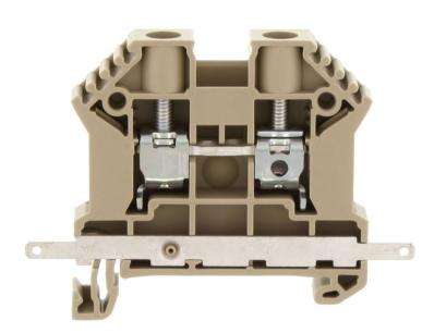
Feed-through terminal, Screw connection, Mounting type: Mounting rail TS 35/7.5, Rated cross-section: 10 mm², Width: 8 mm, Colour: Black
