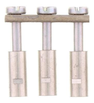
Cross-connector, No. of poles: 3, Mounting type: Can be screwed on, Width: 22.2 mm, Rated cross-section: 10 mm², Colour: natural
