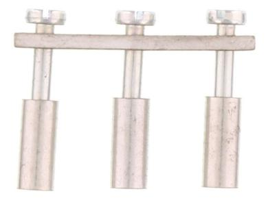
Cross-connector, No. of poles: 3, Mounting type: Can be screwed on, Width: 32 mm, Rated cross-section: 16 mm<sup>2</sup>, Colour: natural
