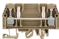
Test disconnect terminal, Screw connection, Mounting type:Mounting rail TS 35/7.5 and TS 32, Rated cross-section: 10 mm<sup>2</sup>, Width: 8 mm, Colour: Beige
