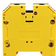
Feed-through terminal, Screw connection, Mounting type: Mounting rail TS 35/7.5, Rated cross-section: 50 mm<sup>2</sup>, Width: 18.5 mm, Colour: Black-yellow
