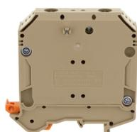
Ex feed-through terminal ATEX-certified, Screw connection, Mounting type:Mounting rail TS 35/7.5 and TS 32, Rated cross-section: 50 mm<sup>2</sup>, Width: 20 mm, Colour: Beige
