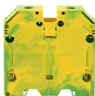
Protective earth terminal, Screw connection, Mounting type: Mounting rail TS 35/7.5, Rated cross-section: 50 mm<sup>2</sup>, Width: 18.5 mm, Colour: Green-yellow
