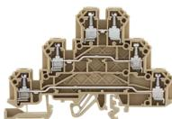
Three-level initiator terminal | Multi-wire terminal, Screw connection, Mounting type:Mounting rail TS 35/7.5 and TS 32, Rated cross-section: 2.5 mm<sup>2</sup>, Width: 5 mm, Colour: Beige
