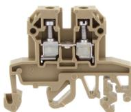
Feed-through terminal, Screw connection, Mounting type: Mounting rail TS 35/7.5 and TS 32, Rated cross-section: 2.5 mm<sup>2</sup>, Width: 5 mm, Colour: Beige
