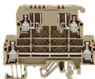
Fuse-disconnect terminal, Screw connection, Mounting type: Mounting rail TS 35/7.5 and TS 32, Rated cross-section: 4 mm<sup>2</sup>, Width: 8 mm, Colour: Beige
