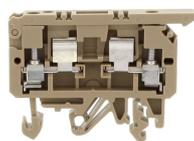
Fuse-disconnect terminal, Screw connection, Mounting type: Mounting rail TS 35/7.5 and TS 32, Rated cross-section: 4 mm<sup>2</sup>, Width: 8 mm, Colour: Beige
