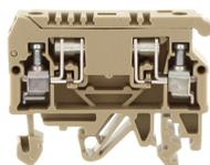
Disconnect terminal, Screw connection, Mounting type: Mounting rail TS 35/7.5 and TS 32, Rated cross-section: 4 mm<sup>2</sup>, Width: 8 mm, Colour: Beige
