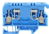
Disconnect terminal, Screw connection, Mounting type: Mounting rail TS 15/5.5, Rated cross-section: 4 mm<sup>2</sup>, Width: 8 mm, Colour: Blue
