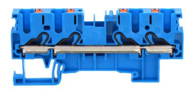
Feed-through terminal, Push-in connection, Mounting type: Mounting rail TS 35/7.5, Rated cross-section: 4 mm², Width: 6.1 mm, Colour: Blue
