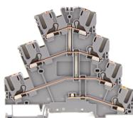
Three-level initiator terminal | Multi-wire terminal, Push-in connection, Mounting type: Mounting rail TS 35/7.5, Rated cross-section: 2.5 mm<sup>2</sup>, Width: 5.1 mm, Colour: Grey
