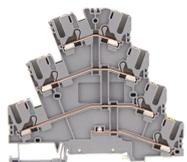
Three-level initiator terminal | Multi-wire terminal, Push-in connection, Mounting type: Mounting rail TS 35/7.5, Rated cross-section: 2.5 mm<sup>2</sup>, Width: 5.1 mm, Colour: Grey
