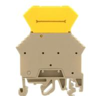
Disconnect terminal, Screw connection, Mounting type:Mounting rail TS 35/7.5 and TS 32, Rated cross-section: 2.5 mm<sup>2</sup>, Width: 6 mm, Colour: Beige
