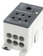
Screw-distributor block, Screw connection, Mounting type:Mounting rail TS 35/7.5 and mounting surface, Rated cross-section of input: 120 mm<sup>2</sup>, Rated cross-section of output: 35 mm<sup>2</sup>, Colour: Dark grey
