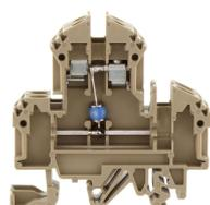
Double-level terminal with electronic components, Screw connection, Mounting type: Mounting rail TS 35/7.5 and TS 32, Rated cross-section: 4 mm<sup>2</sup>, Width: 12 mm, Colour: Beige
