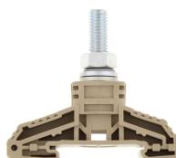
High-power stud terminal, Stud connection, Mounting type: Mounting rail TS 35/7.5, Rated cross-section: 50 mm<sup>2</sup>, Width: 21 mm, Colour: Beige
