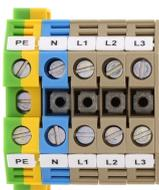
Five-wire mains-connection block, Screw connection, Mounting type: Mounting rail TS 35/7.5 and TS 32, Rated cross-section: 10 mm<sup>2</sup>, Colour: Multi-coloured
