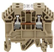
Terminal block for temperature measuring circuits, Screw connection, Mounting type: Mounting rail TS 35/7.5 and TS 32, Rated cross-section: 2.5 mm<sup>2</sup>, Width: 10 mm, Colour: Beige
