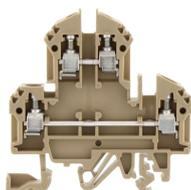
Ex double-level terminal ATEX-certified, Screw connection, Mounting type: Mounting rail TS 35/7.5 and TS 32, Rated cross-section: 4 mm<sup>2</sup>, Width: 5 mm, Colour: Beige
