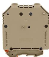
Ex feed-through terminal ATEX-certified, Screw connection, Mounting type: Mounting rail TS 35/7.5 and TS 32, Rated cross-section: 150 mm<sup>2</sup>, Width: 31 mm, Colour: Beige
