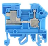
Neutral-disconnect terminal, Screw connection, Mounting type:Mounting rail TS 35/7.5 and TS 32, Rated cross-section: 4 mm<sup>2</sup>, Width: 6 mm, Colour: Blue
