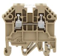
Terminal block for temperature measuring circuits, Screw connection, Mounting type: Mounting rail TS 35/7.5 and TS 32, Rated cross-section: 2.5 mm<sup>2</sup>, Width: 10 mm, Colour: Beige
