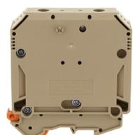
Feed-through terminal, Screw connection, Mounting type: Mounting rail TS 35/7.5 and TS 32, Rated cross-section: 95 mm<sup>2</sup>, Width: 25 mm, Colour: Beige
