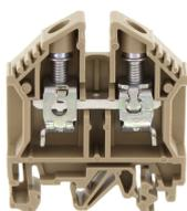
Ex feed-through terminal ATEX-certified, Screw connection, Mounting type:Mounting rail TS 35/7.5 and TS 32, Rated cross-section: 16 mm<sup>2</sup>, Width: 12 mm, Colour: Beige
