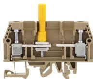
Test disconnect terminal, Screw connection, Mounting type:Mounting rail TS 35/7.5 and TS 32, Rated cross-section: 10 mm<sup>2</sup>, Width: 8 mm, Colour: Beige
