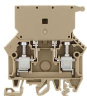
Fuse-disconnect terminal, Screw connection, Mounting type: Mounting rail TS 35/7.5 and TS 32, Rated cross-section: 10 mm<sup>2</sup>, Width: 8 mm, Colour: Beige
