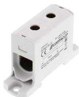
Screw-distributor block, Screw connection, Mounting type: Mounting rail TS 35/7.5 and mounting surface, Rated cross-section of input: 95 mm<sup>2</sup>, Rated cross-section of output: 95 mm<sup>2</sup>, Colour: Light grey
