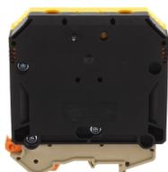
Feed-through terminal, Screw connection, Mounting type: Mounting rail TS 35/7.5 and TS 32, Rated cross-section: 95 mm<sup>2</sup>, Width: 25 mm, Colour: Black-yellow
