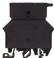
Fused terminal with disconnect plug, Screw connection, Mounting type:Mounting rail TS 35/7.5 and TS 32, Rated cross-section: 10 mm<sup>2</sup>, Width: 10 mm, Colour: Black
