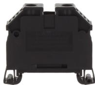
Feed-through terminal, Screw connection, Mounting type: Mounting rail TS 35/7.5, Rated cross-section: 16 mm<sup>2</sup>, Width: 12 mm, Colour: Black
