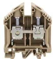
Feed-through terminal, Screw connection, Mounting type:Mounting rail TS 35/7.5 and TS 32, Rated cross-section: 35 mm<sup>2</sup>, Width: 16 mm, Colour: Beige
