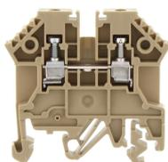
Ex feed-through terminal ATEX-certified, Screw connection, Mounting type:Mounting rail TS 35/7.5 and TS 32, Rated cross-section: 2.5 mm<sup>2</sup>, Width: 5 mm, Colour: Beige
