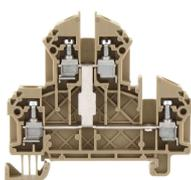
Double-level terminal, Screw connection, Mounting type: Mounting rail TS 35/7.5, Rated cross-section: 2.5 mm<sup>2</sup>, Width: 5 mm, Colour: Beige
