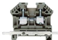
Feed-through terminal, Screw connection, Mounting type: Mounting rail TS 35/7.5, Rated cross-section: 4 mm<sup>2</sup>, Width: 6 mm, Colour: Beige
