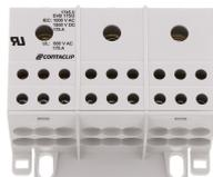
Screw-distributor block, Screw connection, Mounting type:Mounting rail TS 35/7.5 and mounting surface, Rated cross-section of input: 70 mm<sup>2</sup>, Rated cross-section of output:16 mm<sup>2</sup>, Colour: Light grey
