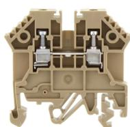
Feed-through terminal, Screw connection, Mounting type: Mounting rail TS 35/7.5, Rated cross-section: 2.5 mm<sup>2</sup>, Width: 5 mm, Colour: Beige
