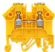
Feed-through terminal, Screw connection, Mounting type: Mounting rail TS 35/7.5 and TS 32, Rated cross-section: 25 mm<sup>2</sup>, Width: 5 mm, Colour: Black-yellow
