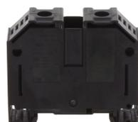
Feed-through terminal, Screw connection, Mounting type: Mounting rail TS 35/7.5, Rated cross-section: 35 mm<sup>2</sup>, Width: 16 mm, Colour: Black
