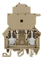
Fuse-disconnect terminal, Screw connection, Mounting type:Mounting rail TS 35/7.5 and TS 32, Rated cross-section: 10 mm<sup>2</sup>, Width: 8 mm, Colour: Beige
