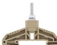
High-power stud terminal, Stud connection, Mounting type: Mounting rail TS 35/7.5, Rated cross-section: 16 mm<sup>2</sup>, Width: 13 mm, Colour: Beige
