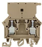
Fused terminal with disconnect plug, Screw connection, Mounting type: Mounting rail TS 35/7.5 and TS 32, Rated cross-section: 10 mm<sup>2</sup>, Width: 8 mm, Colour: Beige
