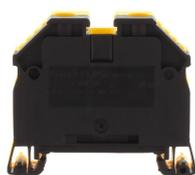
Feed-through terminal, Screw connection, Mounting type: Mounting rail TS 35/7.5, Rated cross-section: 16 mm<sup>2</sup>, Width: 12 mm, Colour: Black-yellow
