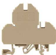
Double-level terminal, Screw connection, Mounting type: Mounting rail TS 35/7.5 and TS 32, Rated cross-section: 4 mm<sup>2</sup>, Width: 7.5 mm, Colour: Beige
