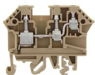
Feed-through terminal, Screw connection, Mounting type: Mounting rail TS 35/7.5 and TS 32, Rated cross-section: 4 mm<sup>2</sup>, Width: 6 mm, Colour: Beige
