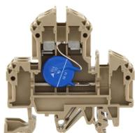
Double-level terminal with electronic components, Screw connection, Mounting type: Mounting rail TS 35/7.5 and TS 32, Rated cross-section: 4 mm<sup>2</sup>, Width: 12 mm, Colour: Beige
