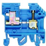
Neutral-disconnect terminal, Screw connection, Mounting type:Mounting rail TS 35/7.5 and TS 32, Rated cross-section: 4 mm<sup>2</sup>, Width: 6 mm, Colour: Blue
