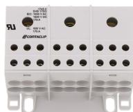
Screw-distributor block, Screw connection, Mounting type:Mounting rail TS 35/7.5 and mounting surface, Rated cross-section of input: 70 mm<sup>2</sup>, Rated cross-section of output: 16 mm<sup>2</sup>, Colour: Light grey
