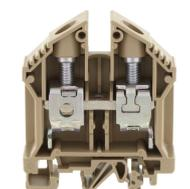
Ex feed-through terminal ATEX-certified, Screw connection, Mounting type: Mounting rail TS 35/7.5 and TS 32, Rated cross-section: 35 mm<sup>2</sup>, Width: 16 mm, Colour: Beige
