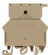
Fused terminal with disconnect plug, Screw connection, Mounting type:Mounting rail TS 35/7.5 and TS 32, Rated cross-section: 10 mm<sup>2</sup>, Width: 10 mm, Colour: Beige
