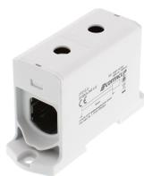
Screw-distributor block, Screw connection, Mounting type:Mounting rail TS 35/7.5 and mounting surface, Rated cross-section of input: 240 mm<sup>2</sup>, Rated cross-section of output: 240 mm<sup>2</sup>, Colour: Light grey
