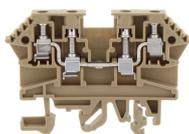
Feed-through terminal, Screw connection, Mounting type: Mounting rail TS 35/7.5 and TS 32, Rated cross-section: 4 mm<sup>2</sup>, Width: 6 mm, Colour: Beige
