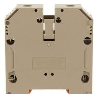
Feed-through terminal, Screw connection, Mounting type: Mounting rail TS 35/7.5, Rated cross-section: 70 mm<sup>2</sup>, Width: 20.5 mm, Colour: Beige
