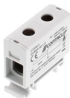
Screw-distributor block, Screw connection, Mounting type:Mounting rail TS 35/7.5 and mounting surface, Rated cross-section of input: 50 mm<sup>2</sup>, Rated cross-section of output: 50 mm<sup>2</sup>, Colour: Light grey
