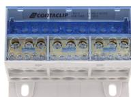
Screw-distributor block, Screw connection, Mounting type:Mounting rail TS 35/7.5 and mounting surface, Rated cross-section of input: 6, 16 and 35 mm<sup>2</sup>, Rated cross-section of output: 6, 16 and 35mm<sup>2</sup>, Colour: Light grey
