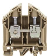
Feed-through terminal, Screw connection, Mounting type: Mounting rail TS 35/7.5 and TS 32, Rated cross-section: 35 mm<sup>2</sup>, Width: 16 mm, Colour: Beige
