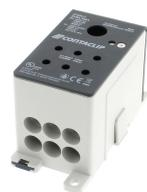
Screw-distributor block, Screw connection, Mounting type:Mounting rail TS 35/7.5 and mounting surface, Rated cross-section of input: 240 mm<sup>2</sup>, Rated cross-section of output: 35 mm<sup>2</sup>, Colour: Dark grey
