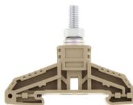
High-power stud terminal, Stud connection, Mounting type: Mounting rail TS 35/7.5, Rated cross-section: 35 mm<sup>2</sup>, Width: 16 mm, Colour: Beige
