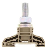
High-power stud terminal, Stud connection, Mounting type: Mounting rail TS 35/7.5, Rated cross-section: 120 mm<sup>2</sup>, Width: 32 mm, Colour: Beige
