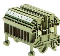
10 terminal feed-through terminal/block variant, Screw connection, Mounting type: Mounting rail TS 35/7.5 and TS 32, Rated cross-section: 2.5 mm<sup>2</sup>, Colour: Beige
