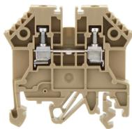
Feed-through terminal, Screw connection, Mounting type:Mounting rail TS 35/7.5, Rated cross-section: 2.5 mm<sup>2</sup>, Width: 5 mm, Colour: Beige
