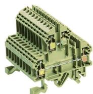
10 terminal double-level terminal/block variant, Screw connection, Mounting type: Mounting rail TS 35/7.5 and TS 32, Rated cross-section: 2.5 mm<sup>2</sup>, Colour: Beige
