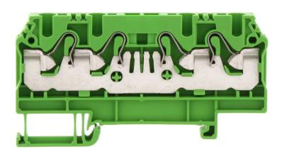
Feed-through terminal, Push-in connection, Mounting type: Mounting rail TS 35/7.5, Rated cross-section: 4 mm², Width: 6.1 mm, Colour: Green
