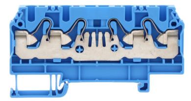
Feed-through terminal, Push-in connection, Mounting type: Mounting rail TS 35/7.5, Rated cross-section: 4 mm<sup>2</sup>, Width: 6.1 mm, Colour: Blue
