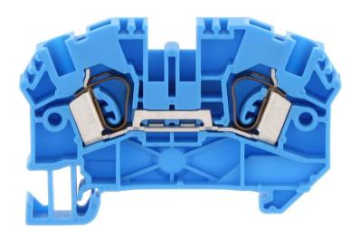
Feed-through terminal, Tension-spring connection, Mounting type: Mounting rail TS 35/7.5, Rated cross-section: 4 mm², Width: 6.1 mm, Colour: Blue
