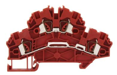
Double-level terminal, Tension-spring connection, Mounting type: Mounting rail TS 35/7.5, Rated cross-section: 2.5 mm<sup>2</sup>, Width: 5.1 mm, Colour: Red
