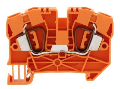
Feed-through terminal, Tension-spring connection, Mounting type: Mounting rail TS 35/7.5, Rated cross-section: 6 mm², Width: 8.1 mm, Colour: Orange
