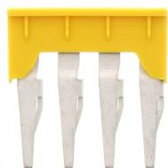
Insulated cross-connector, No. of poles: 4, Mounting type: Plug in, Width: 31.9 mm, Rated cross-section: 6 mm<sup>2</sup>, Colour: Yellow
