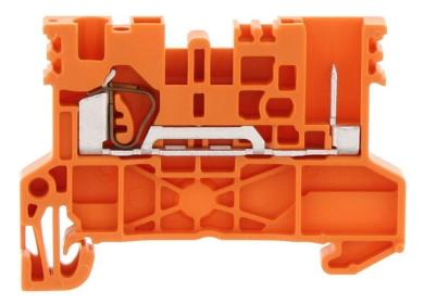
Feed-through terminal, Tension-spring connection, Mounting type: Mounting rail TS 35/7.5, Rated cross-section: 2.5 mm<sup>2</sup>, Width: 5.1 mm, Colour: Orange
