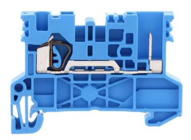
Feed-through terminal, Tension-spring connection, Mounting type: Mounting rail TS 35/7.5, Rated cross-section: 2.5 mm², Width: 5.1 mm, Colour: Blue
