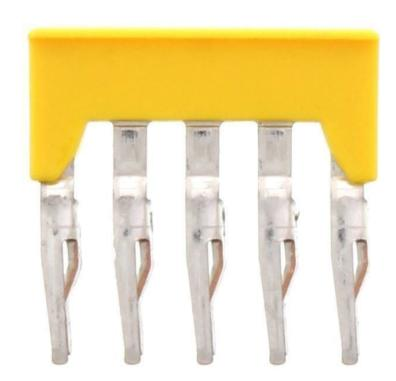
Insulated cross-connector, No. of poles: 5, Mounting type: Plug in, Width: 24.4 mm, Rated cross-section: 2.5 mm², Colour: Yellow
