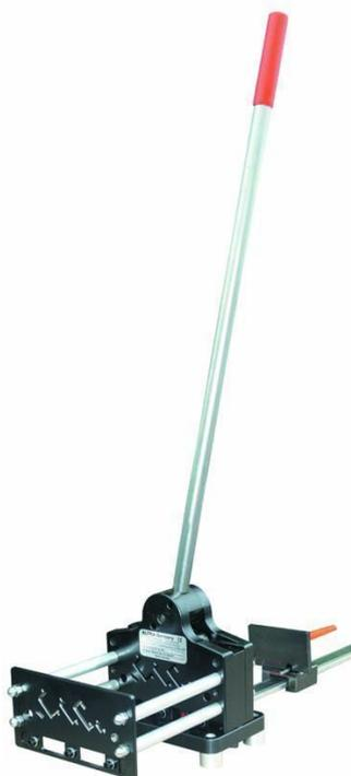
The TS-PSS 2 DIN rail cutter and punching tool is designed for manually shortening and punching holes in DIN rails (TS 15, TS 35, TS 32) and busbars (10 x 3 mm). The tool can be mounted on a workbench or similar working surface. It can also punch holes of varying dimensions in customized positions. A cross-hole/slotted-hole punch (12 x 6.4 mm) is included in the delivery.
