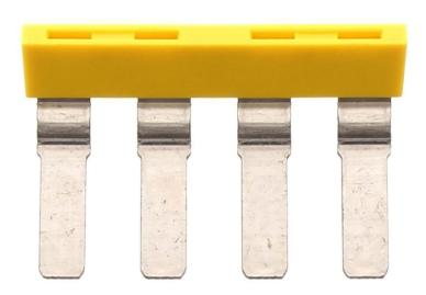
External insulated cross-connector, No. of poles: 4, Mounting type: Plug in, Width: 38.3 mm, Rated current: 57 A; Colour: Yellow
