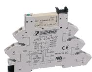
Plug-Relay-Compact (PRC) Complete, Consisting of base PRC... with tension-spring connection and pluggable miniature relay PRC... with multi-layer gold contact, Mounting type: Mounting rail TS 35, 1 CO contact, Input voltage: 24 VDC
