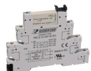
Plug-Relay-Compact (PRC) Complete, Consisting of base PRC... with screw connection and pluggable miniature relay PRC... with power contact, Mounting type: Mounting rail TS 35, 1 CO contact, Input voltage: 24 VAC/DC
