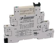
Plug-Relay-Compact (PRC) Complete, Consisting of base PRC... with screw connection and pluggable miniature relay PRC... with power contact, Mounting type: Mounting rail TS 35, 1 CO contact, Input voltage: 48 VAC/DC
