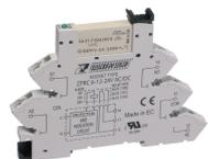
Plug-Relay-Compact (PRC) socket base PRC with tension-spring connection and residual current suppression for long cables, Mounting type: Mounting rail TS 35, 1 CO contact, Input voltage: 110 to 125 VAC/DC
