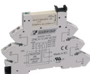
Plug-Relay-Compact (PRC) Complete, Consisting of base PRC... with tension-spring connection and pluggable miniature relay PRC... with power contact, Mounting type: Mounting rail TS 35, 1 CO contact, Input voltage: 240 VAC/DC
