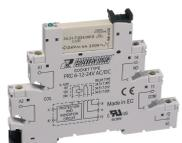
Plug-Relay-Compact (PRC) socket base PRC with screw connection, Mounting type: Mounting rail TS 35, 1 CO contact, Input voltage: 230 to 240 VAC
