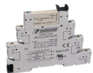
Plug-Relay-Compact (PRC) socket base PRC with screw connection and residual current suppression for long cables, Mounting type: Mounting rail TS 35, 1 CO contact, Input voltage: 110 to 125 VAC/DC
