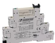
Plug-Relay-Compact (PRC) socket base PRC with screw connection and residual current suppression for long cables, Mounting type: Mounting rail TS 35, 1 CO contact, Input voltage: 220 to 240 VAC
