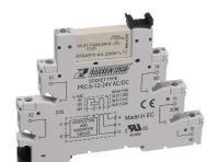
Plug-Relay-Compact (PRC) Complete, Consisting of base PRC... with screw connection and pluggable miniature relay PRC... with power contact, Mounting type: Mounting rail TS 35, 1 CO contact, Input voltage: 125 VAC/DC
