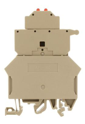
Fuse-disconnect terminal, Screw connection, Mounting type:Mounting rail TS 35/7.5 and TS 32, Rated cross-section: 10 mm², Width: 10 mm, Colour: Beige
