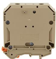
Feed-through terminal, Screw connection, Mounting type: Mounting rail TS 35/7.5 and TS 32, Rated cross-section: 95 mm<sup>2</sup>, Width: 25 mm, Colour: Beige
