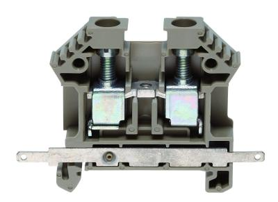
Feed-through terminal, Screw connection, Mounting type: Mounting rail TS 35/7.5, Rated cross-section: 10 mm², Width: 8 mm, Colour: Beige
