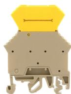
Disconnect terminal, Screw connection, Mounting type: Mounting rail TS 35/7.5 and TS 32, Rated cross-section: 2.5 mm<sup>2</sup>, Width: 6 mm, Colour: Beige
