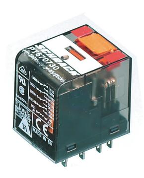
Plug-in industrial relays with power contacts, 4 CO contacts, Test button, Mechanical switching position indicator, Input voltage: 115 VAC
