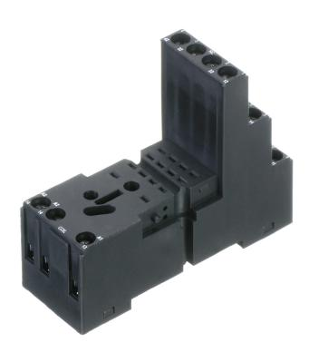
Relay socket base PRS, for industrial relay with 4 CO contacts, Screw connection, Plug-in option for input/suppression modules, Mounting type: Mounting rail TS 35
