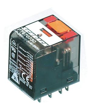
Plug-in industrial relays with power contacts, 4 CO contacts, Test button, Mechanical switching position indicator, Input voltage: 12 VAC
