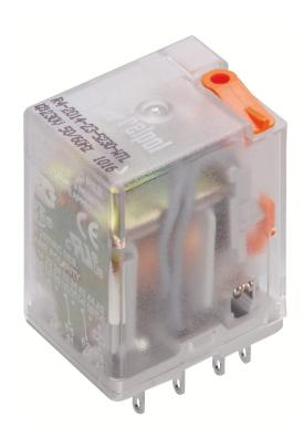
Plug-in industrial relays with power contacts, 2 CO contacts, Test button, Status LED, Mechanical switching position indicator, Input voltage: 230 VAC
