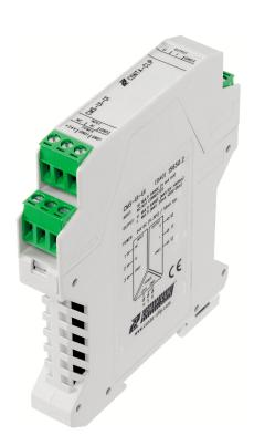
Signal converter for converting voltage/current signals to an analogue standard signal, 3-way electrical isolation, Screw connection, Mounting type: Mounting rail TS 35, Supply voltage: 24 VDC
