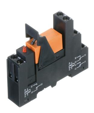
Pre-assembled relay module PRS..., Screw connection, Consisting of: relay socket base, power contact relay, pluggable display/suppression module and holding clip, 2 CO contacts, Input voltage: 110 VDC
