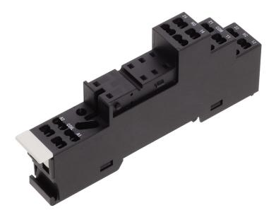
Relay socket base PRS, for miniature power relay with 2 CO contacts, Tension-spring connection, Plug-in option for input/suppression modules, Mounting type: Mounting rail TS 35
