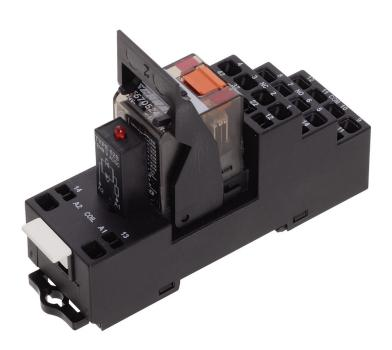
Pre-assembled relay module PRS..., Tension-spring connection, Consisting of: relay socket base, power contact relay, pluggable display/suppression module and holding clip, 4 CO contact, Input voltage: 60 VDC
