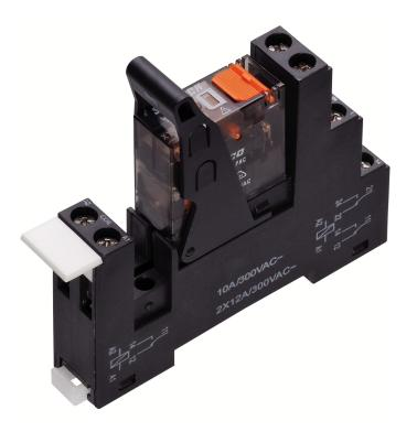
Pre-assembled relay module PRSXT, Screw connection, Consisting of: relay socket, holding clip and power contact relay with test button and status LED. 2 CO contacts, Input voltage: 24 VAC
